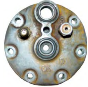
GK SD7 Rear Vert. Pad with schrader & blowoff
