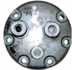
MJ SD7 Rear Horiz. Tube & O with blowoff
