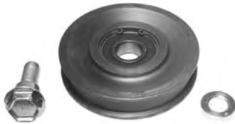
Back Side Idler 3 5/8" Dia x 3/4" wide, 17/32" groove width x 1/8" groove depth.
