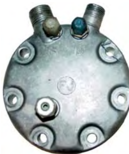
FJ SD7 Vert. O-ring with schraders & blowoff
